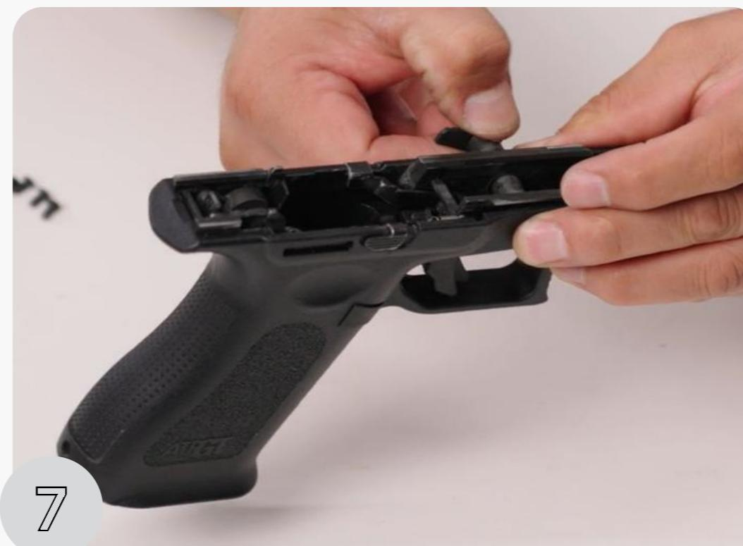
07 Then directly pull the take down lever from the left side of the frame.
