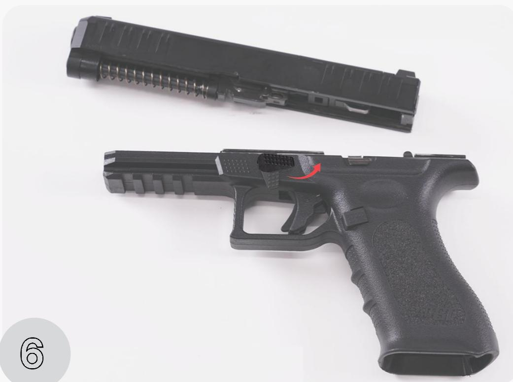
06 Turn the take down lever counter clockwise 90 degrees, back to the original position.
