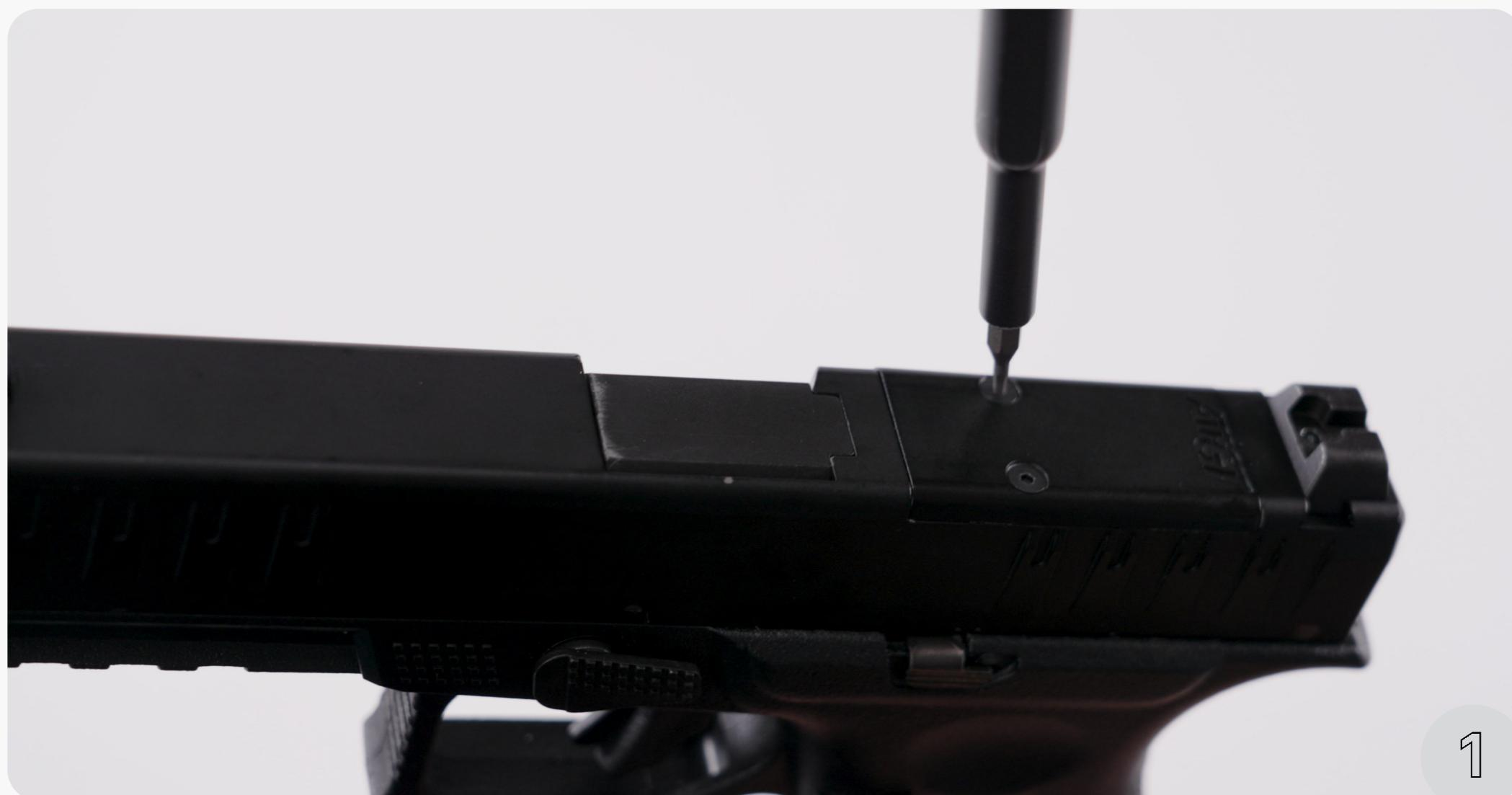
01 Unscrew both screws from the top of the cover plate to remove the cover plate.
