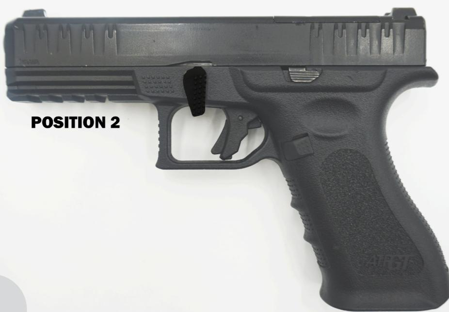
04 Turn the take down lever from the left side of the frame clockwise 90 degrees.
