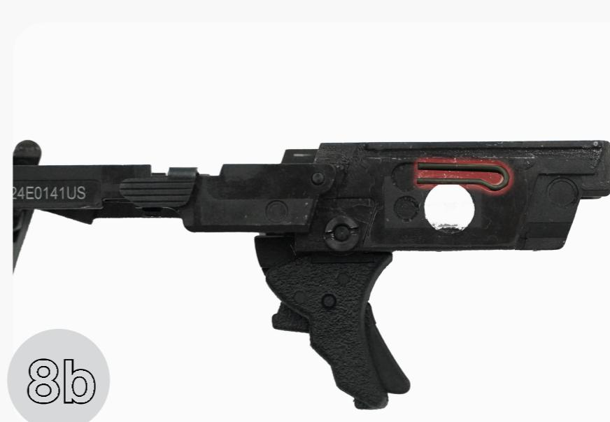
\* **Warning:** Pay attention to the Lock in spring, it will easily drop while removing the Trigger group unit\*
